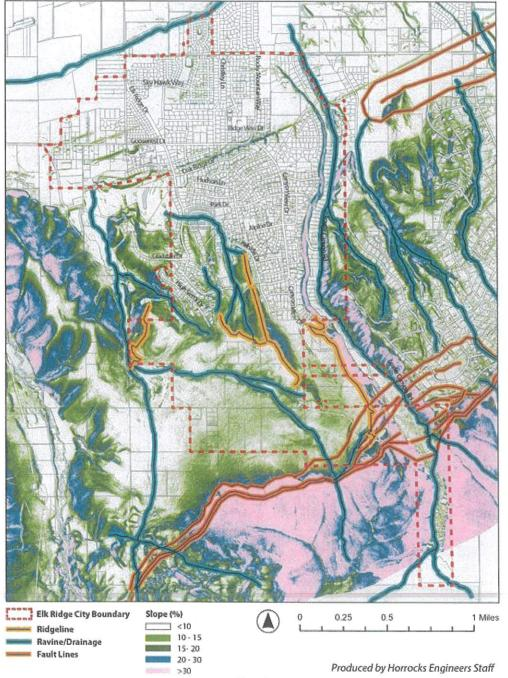
Slope data source: 0.5 Meter LIDAR data captured in 2013-2014 taken from the Utah Geospatial Resource Center (UGRC) website. This is the most recent and accurate data available.
